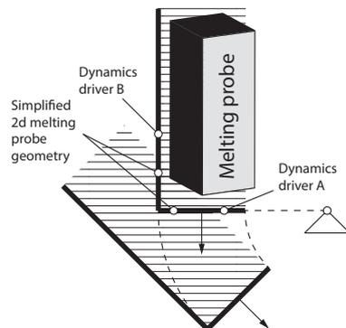
Figure: Schematic of the 2d curvilinear melting method applied to a 3d melting probe.
